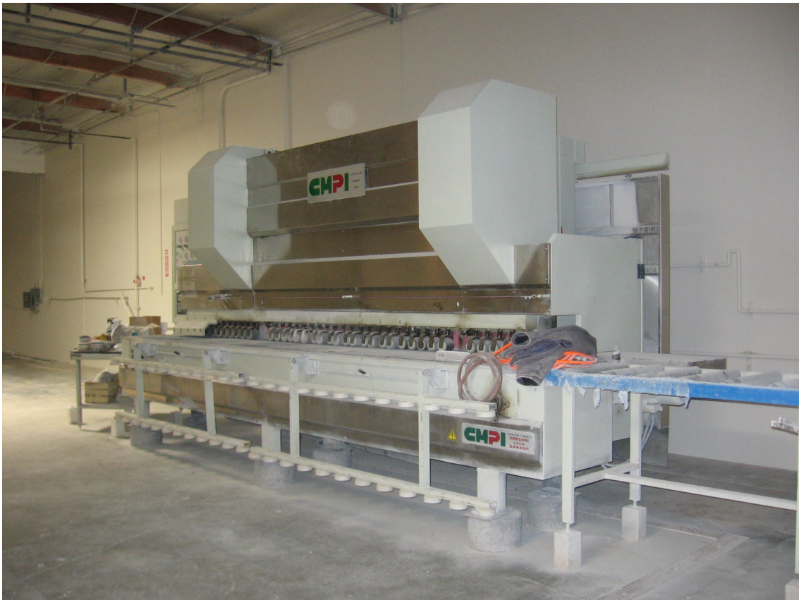
Photograph 6 - Stone cutting machine inside warehouse
