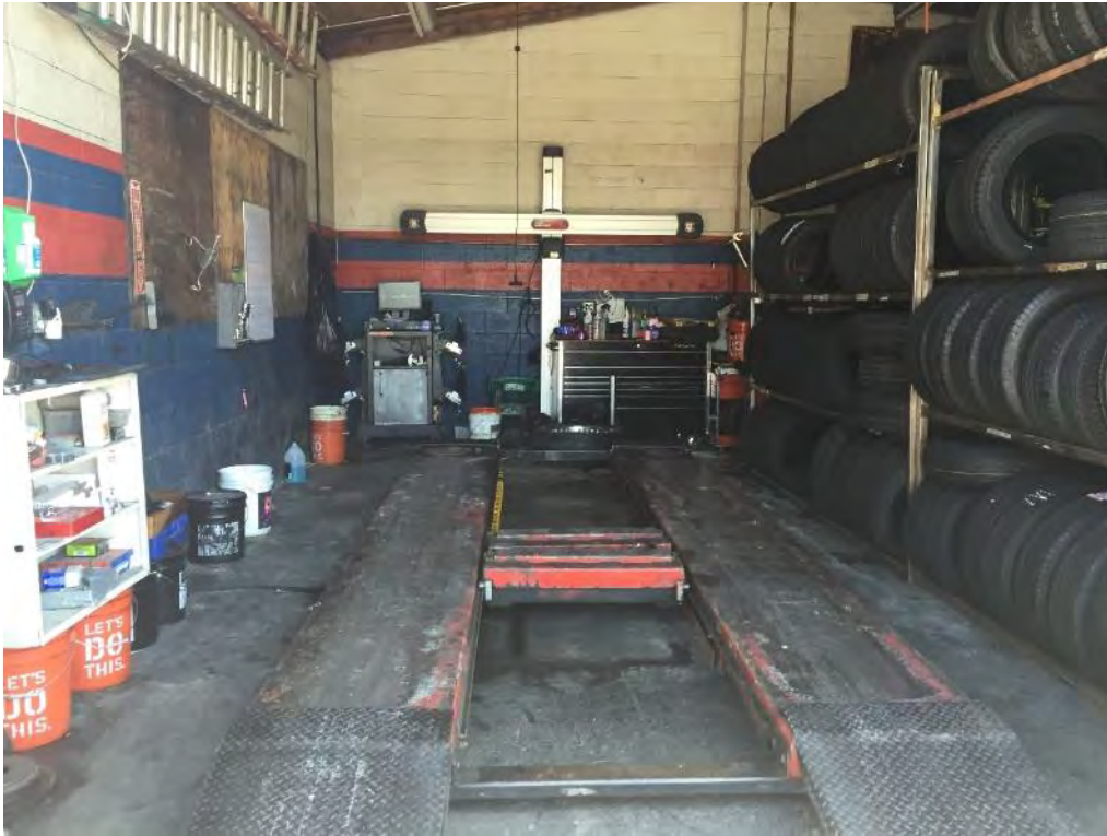
Photograph 11. In-ground lift located within the interior of the tire shop.
