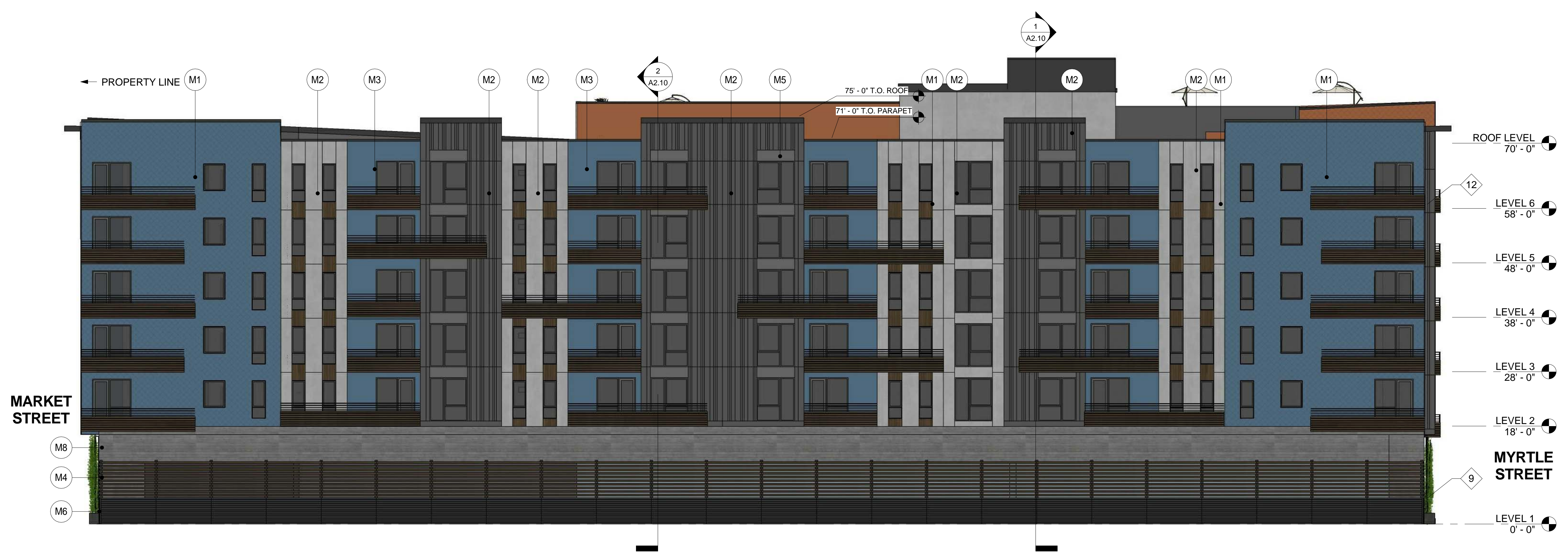
2 EXTERIOR ELEVATION - NORTH 3/32" = 1'-0"
