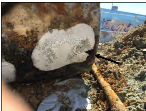
Photograph 5: The third UST was found in poor condition with a 4-inch diameter hole.
