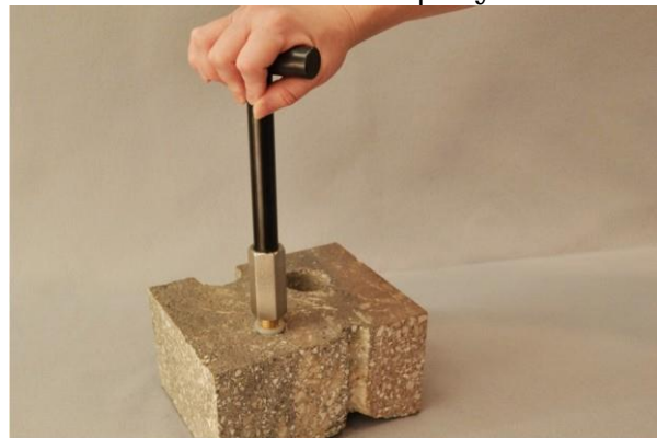
Figure 7. Removing the VAPOR PIN®
