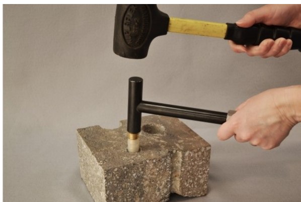
Figure 2. Installing the Vapor Pin™.
