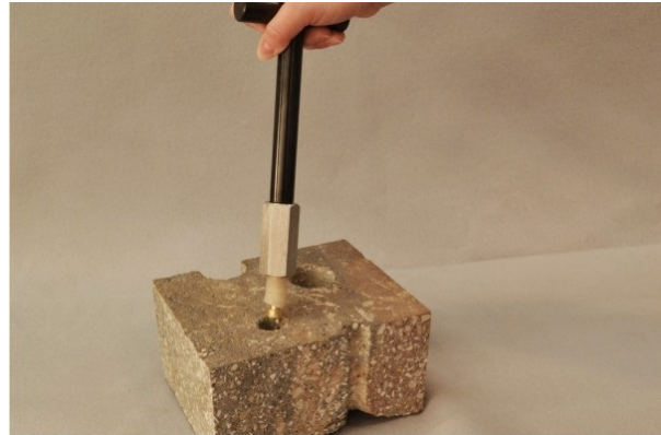
Figure 8. Extracted Vapor Pin™.
