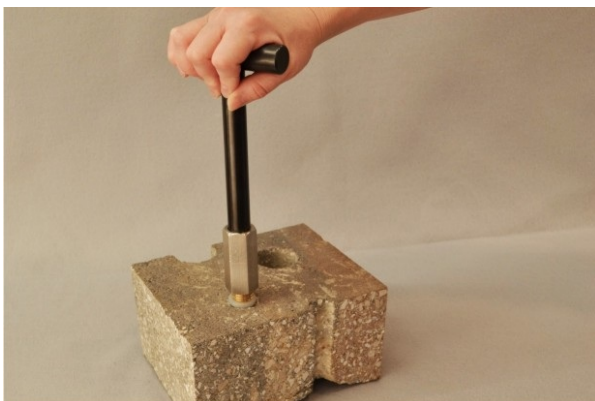
Figure 7. Removing the Vapor Pin™.
