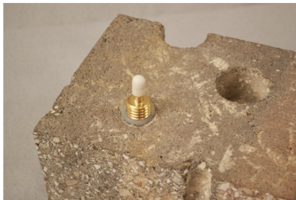
Figure 4. Installed Vapor Pin™.
