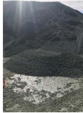
3/4-inch Class 2 Aggregate Base (AB) Stockpile at the Cemex Clayton Quarry. Twelve (12) 4-point composite samples were collected from a representative stockpile of the 3/4-inch AB; six samples submitted for asbestos analysis and six samples submitted for the remaining analyses.
