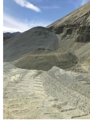
1/2-inch Dust Tailings (DT) Stockpile at the Cemex Clayton Quarry. Twelve (12) 4-point composite samples were collected from a representative stockpile of the 1/2-inch Dust Tailings; six samples submitted for asbestos analysis and six samples submitted for the remaining analyses.
