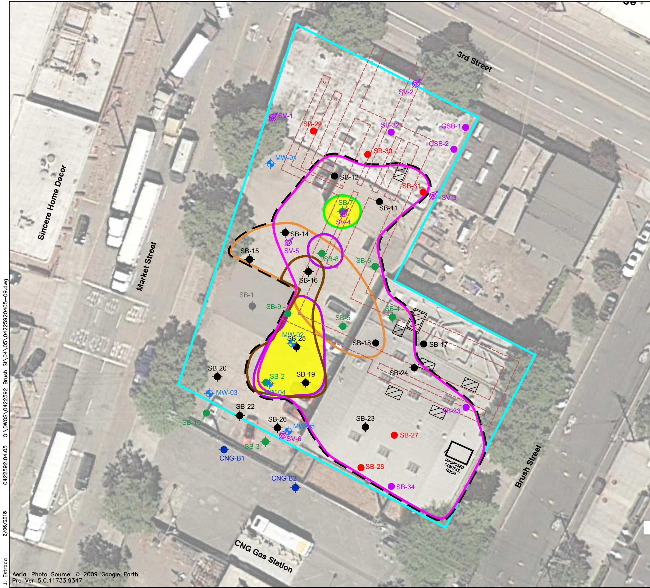
Figure 3 Areas to Be Excavated to the Dewatered Water Table Construction Soil and Groundwater Management Plan 205 Brush Street Oakland, California
