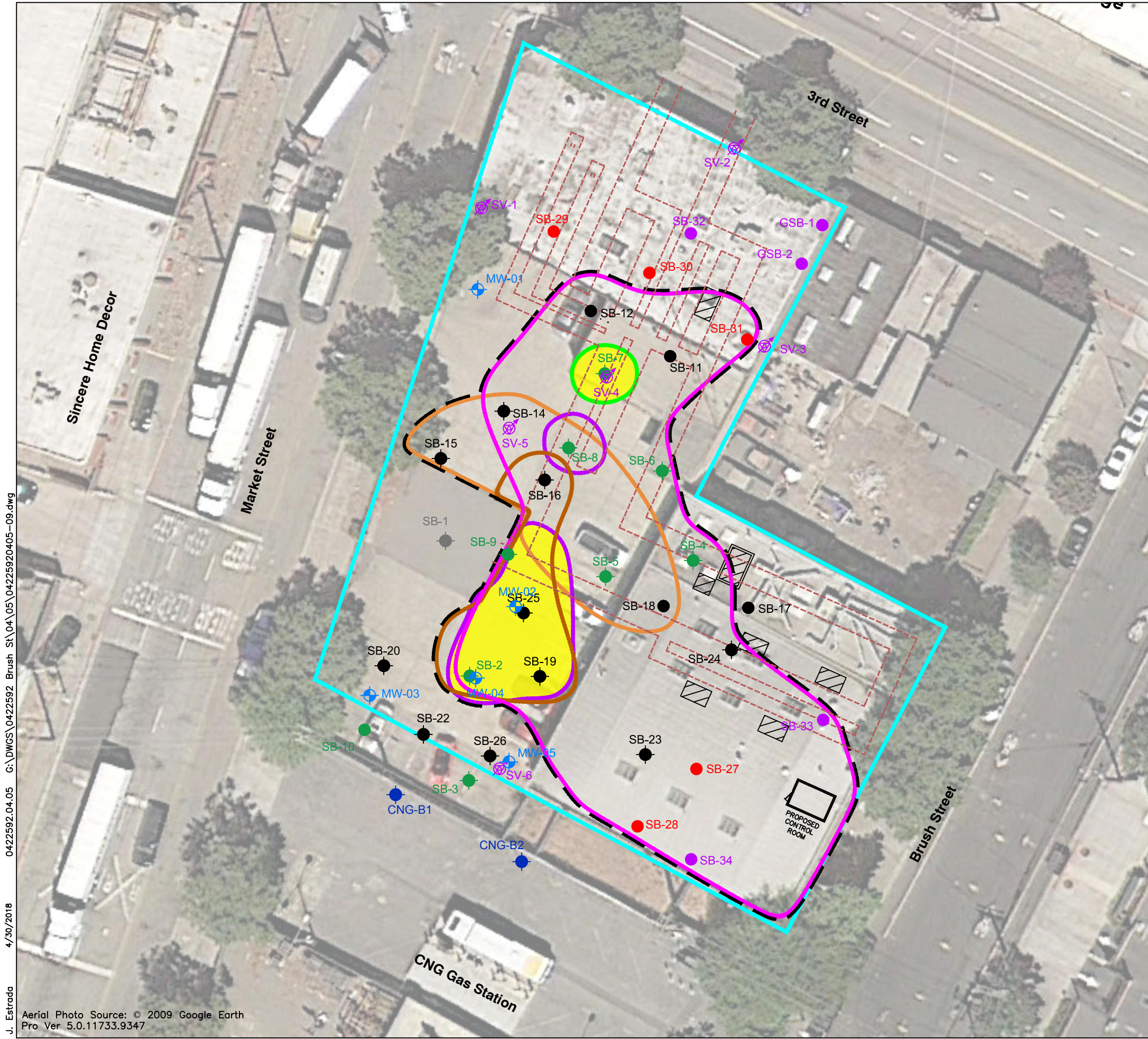
Figure 2 Remediation Excavation Areas and Trench Areas Soil Import Management Plan 205 Brush Street Oakland, California
