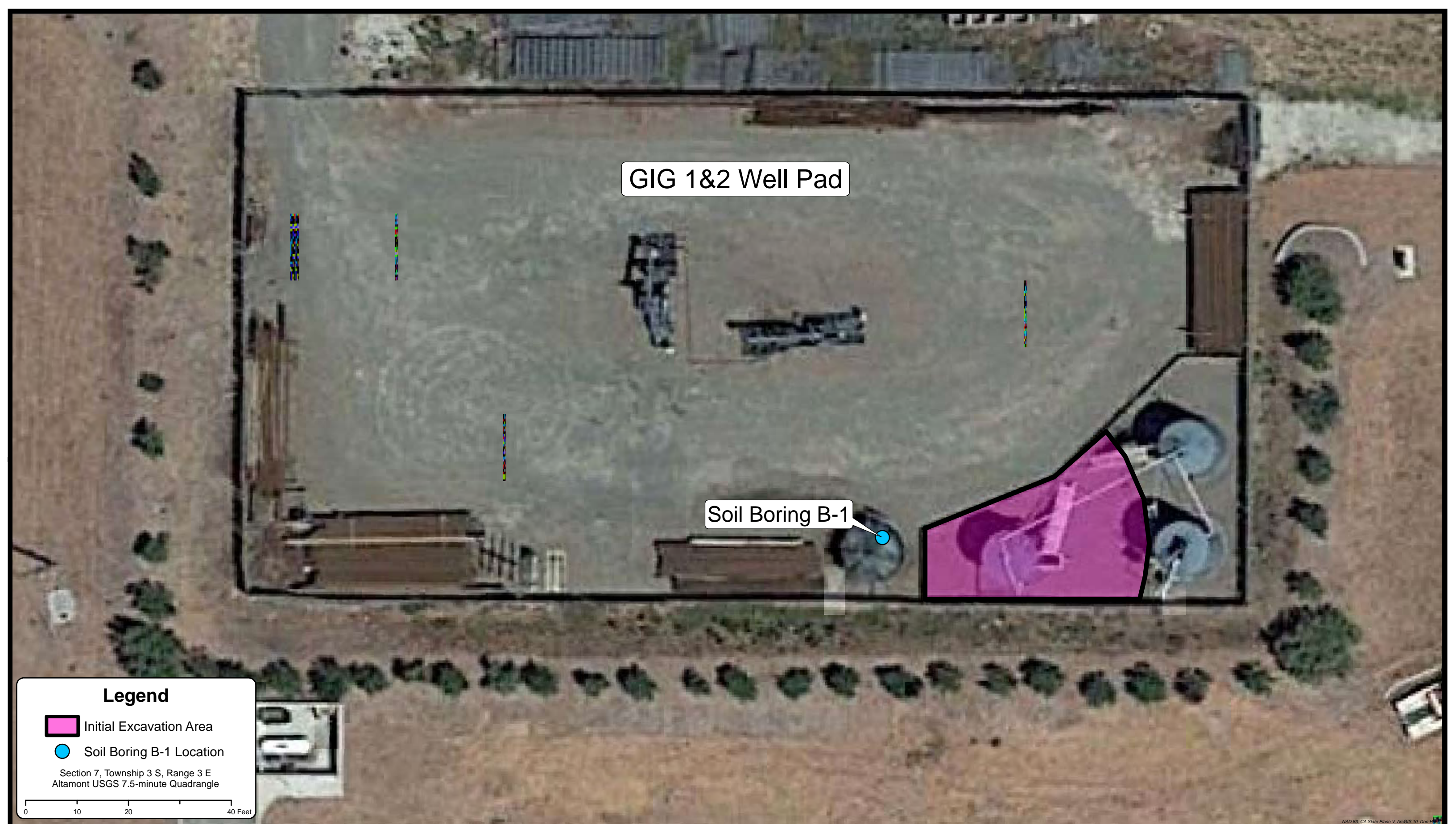
FIGURE 2 Initial Excavation Limits and Soil Boring B-1
