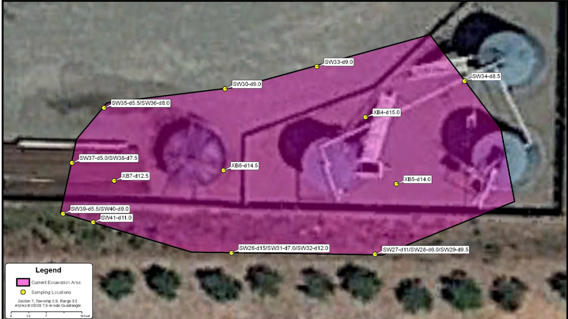
FIGURE 4 Former GIG Tank Facility Excavation and Sample Locations
