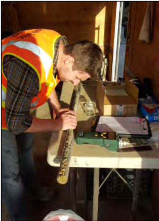
Photograph 3: The plastic cores from the Geoprobe rig were cut open for geological logging.
