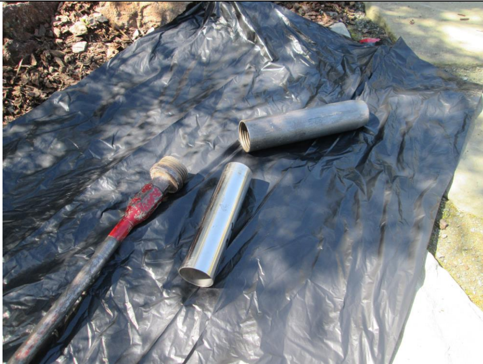
Subject : Drive hammer sampling apparatus used for soil collection
