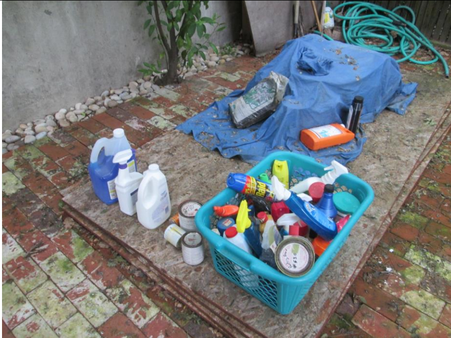
Subject: Basement room household chemicals removed to outside garden before indoor air survey
