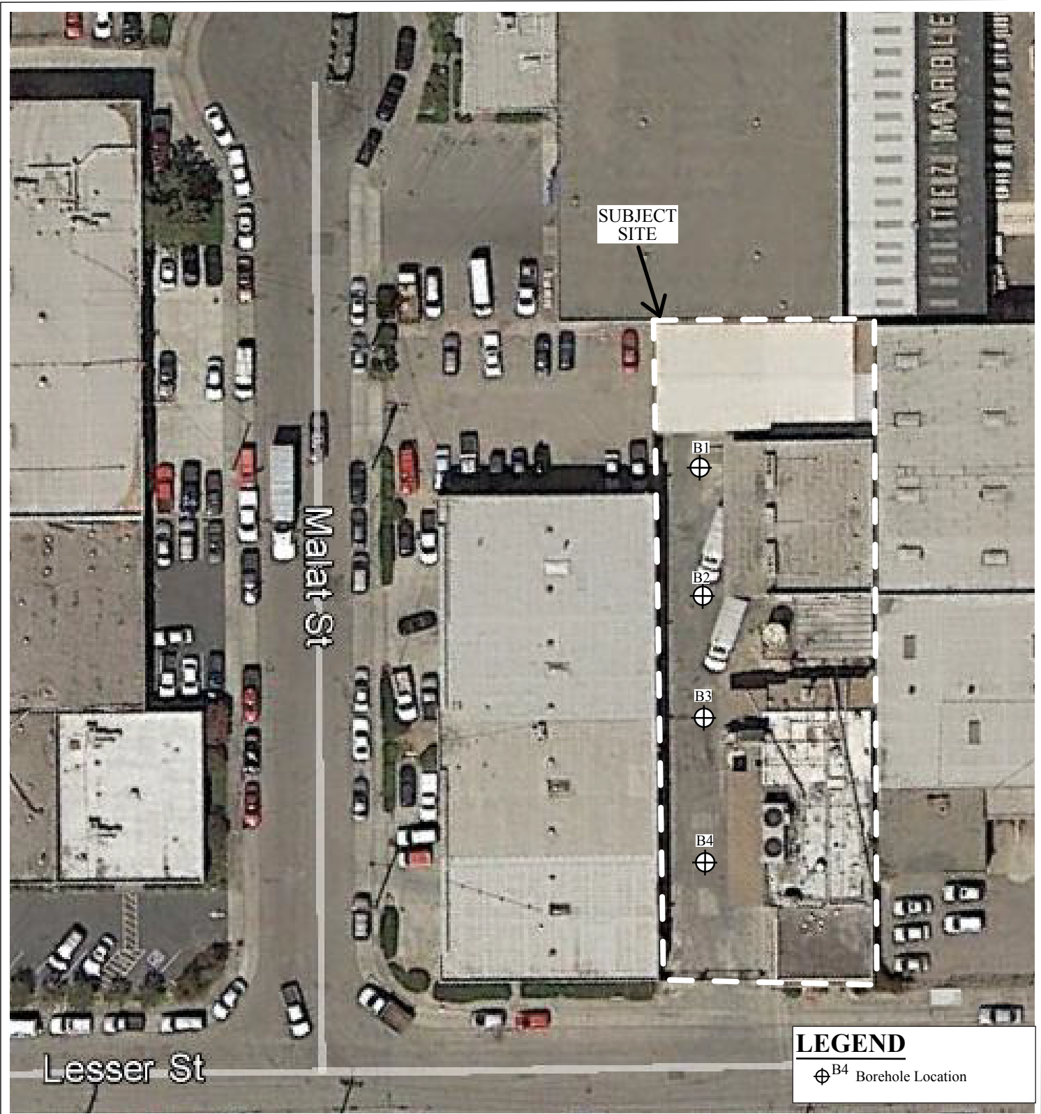
Figure 2 Site Aerial Photograph Showing Borehole Locations 475 Lesser Street Oakland, California
