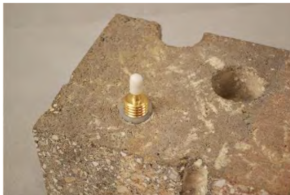
Figure 4. Installed Vapor Pin™.
