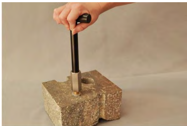
Figure 7. Removing the Vapor Pin™.
