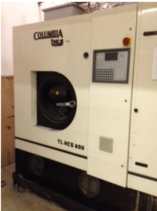
Photo 13: Hydrocarbon Dry Cleaner 7104 Dublin Blvd
