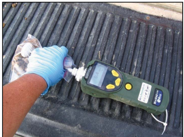
Photograph 2: Soil was screened for VOCs during the well installation and excavations using a PID.
