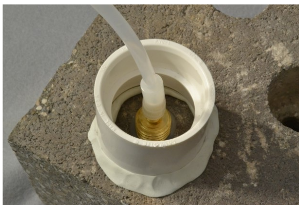
Figure 6. Water dam used for leak detection.
