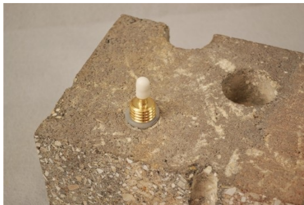
Figure 4. Installed Vapor Pin™.
