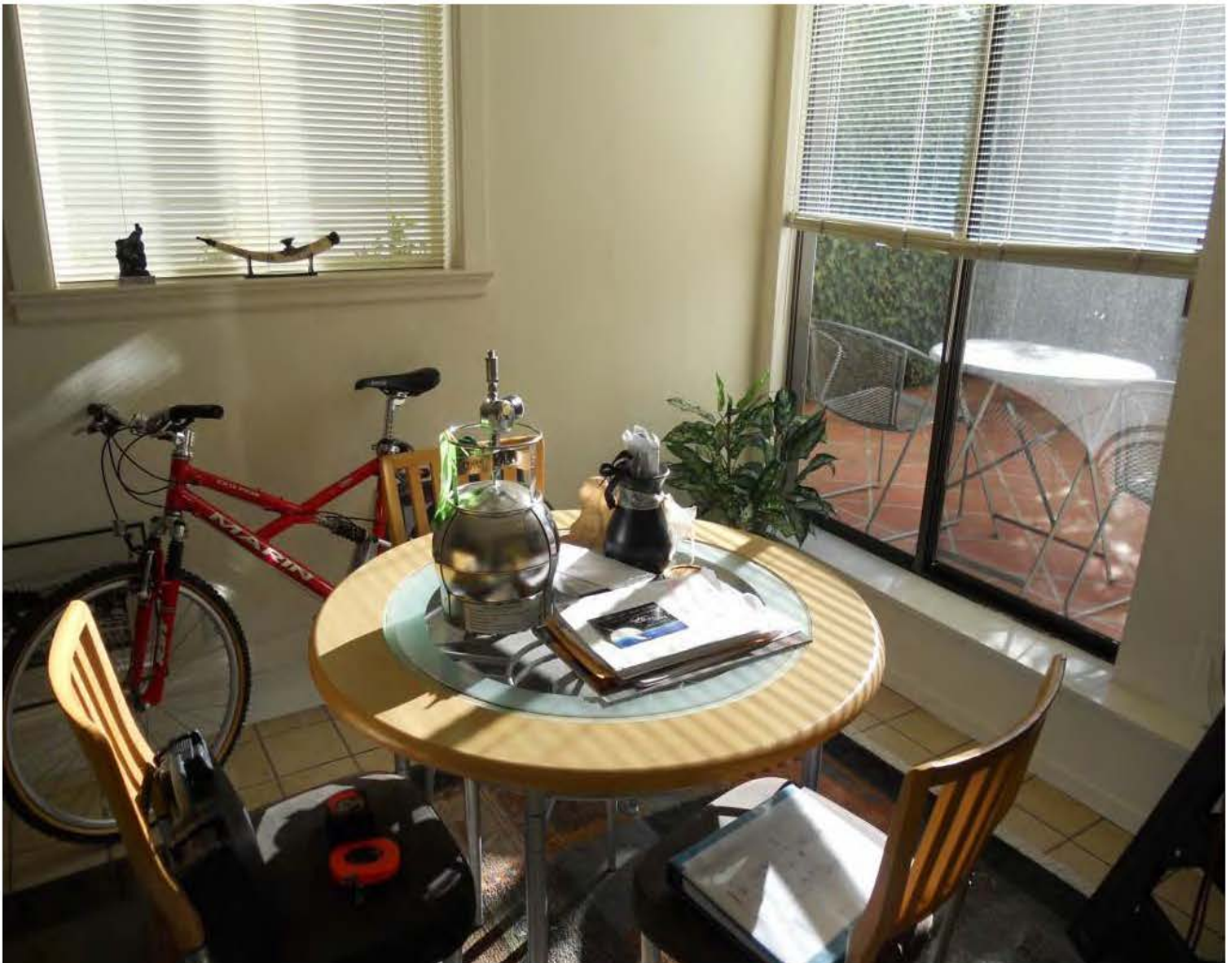
Indoor air sampling canister in use.
