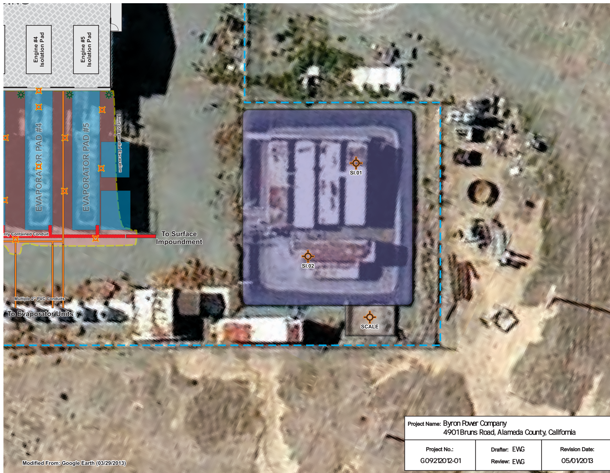
FIGURE 2 SITE MAP DEPICTING SLUDGE AND SCALE DEPOSIT SAMPLE LOCATIONS
