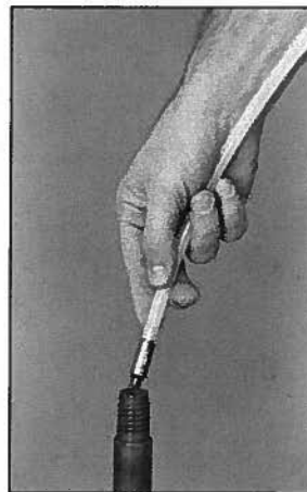
Figure 2. Insertion of tubing and PRT adapter.
