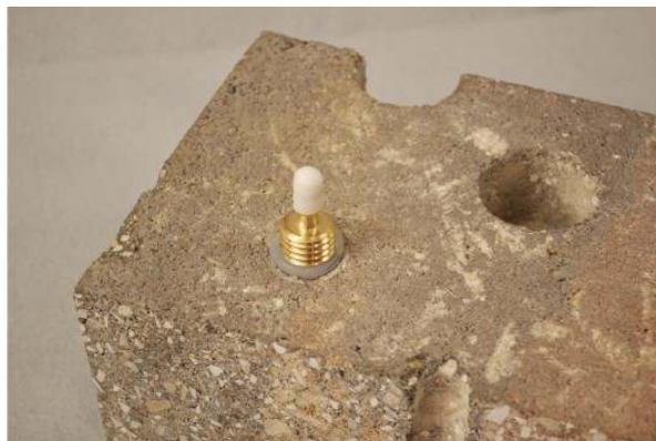
Figure 4. Installed Vapor Pin™.
