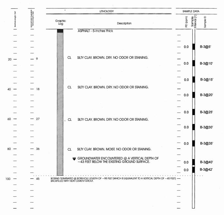
Date Drilled: 7-23-2010 Driller: RSI Drilling Drilling Method: Sonic Boring Angle (2): 30 Degrees Logged By: Derek Wong
