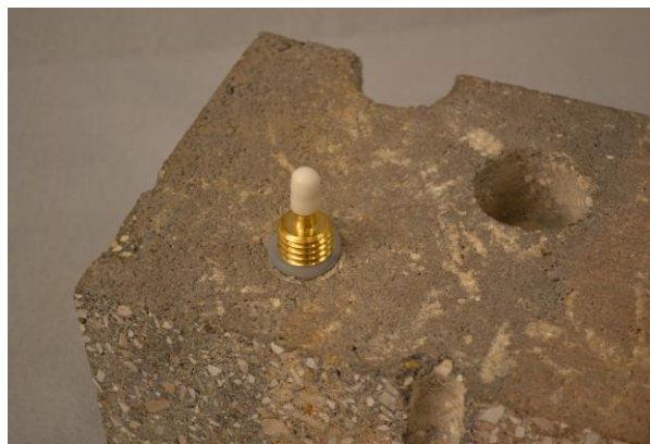
Figure 3. Installed Vapor Pin™
