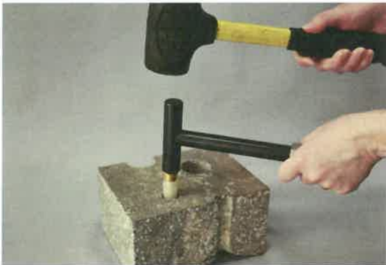
Figure 2. Installing the Vapor Pin™.
