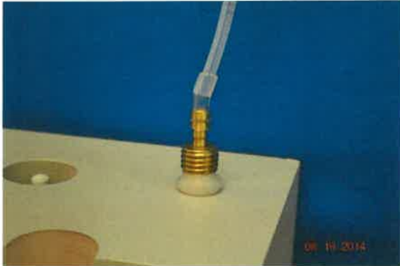
Figure 5. Vapor Pin™ sample connection.
