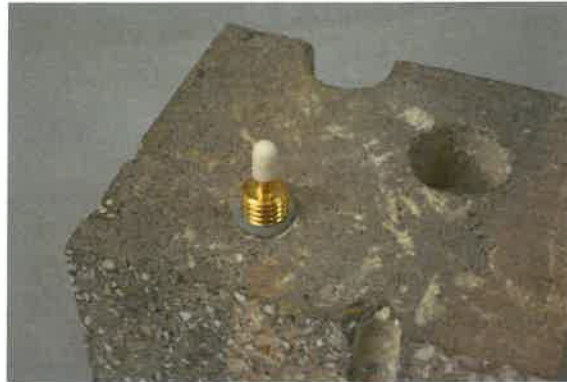
Figure 3. Installed Vapor Pin™
