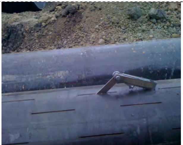
Photograph 5 - Well screen with 0.060 feeler gauge in factory cut perforation.
