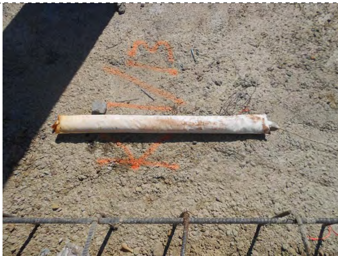
Photograph 5 - This is the full length of the material on August 16, 2012. Discoloration, but for tip, is from rust in the well.
