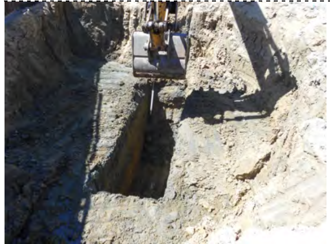
Photograph 22 - A small amount of groundwater accumulated in the trench. Note disposable bailer attached to tooth of excavator being lowered in an effort to collect groundwater sample.
