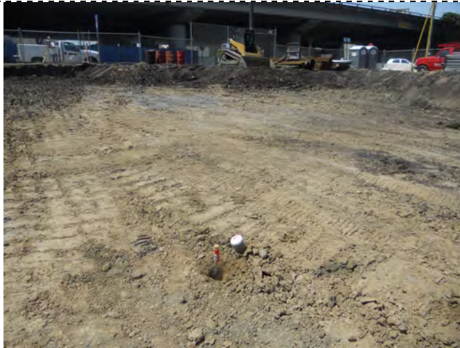
Photograph 1 - Sample C6 was the only confirmation sample collected with significant TPH contamination.
