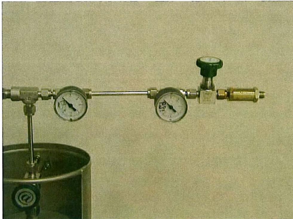
Plate 2: Flow regulator with built-in vacuum gauge connected to the tee fitting.
