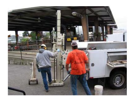
Subject: Drilling at location BH-01 for the collection of soil and groundwater samples.
