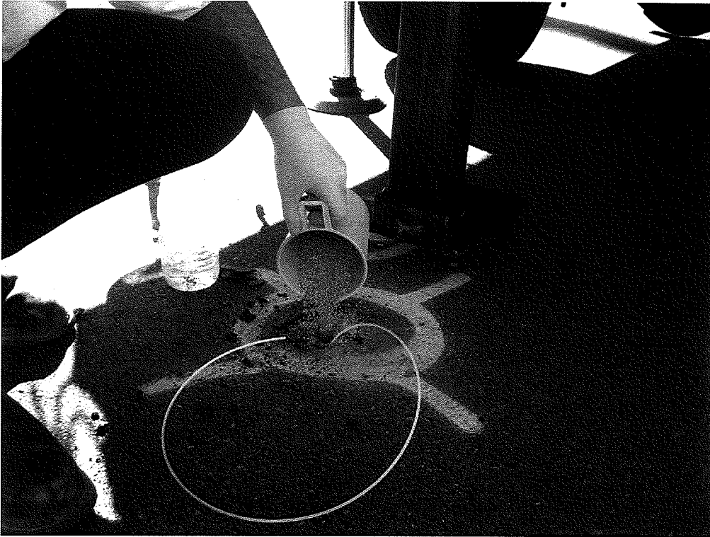
Photo 5, Placing bentonite seal at a soil-gas sampling location.
