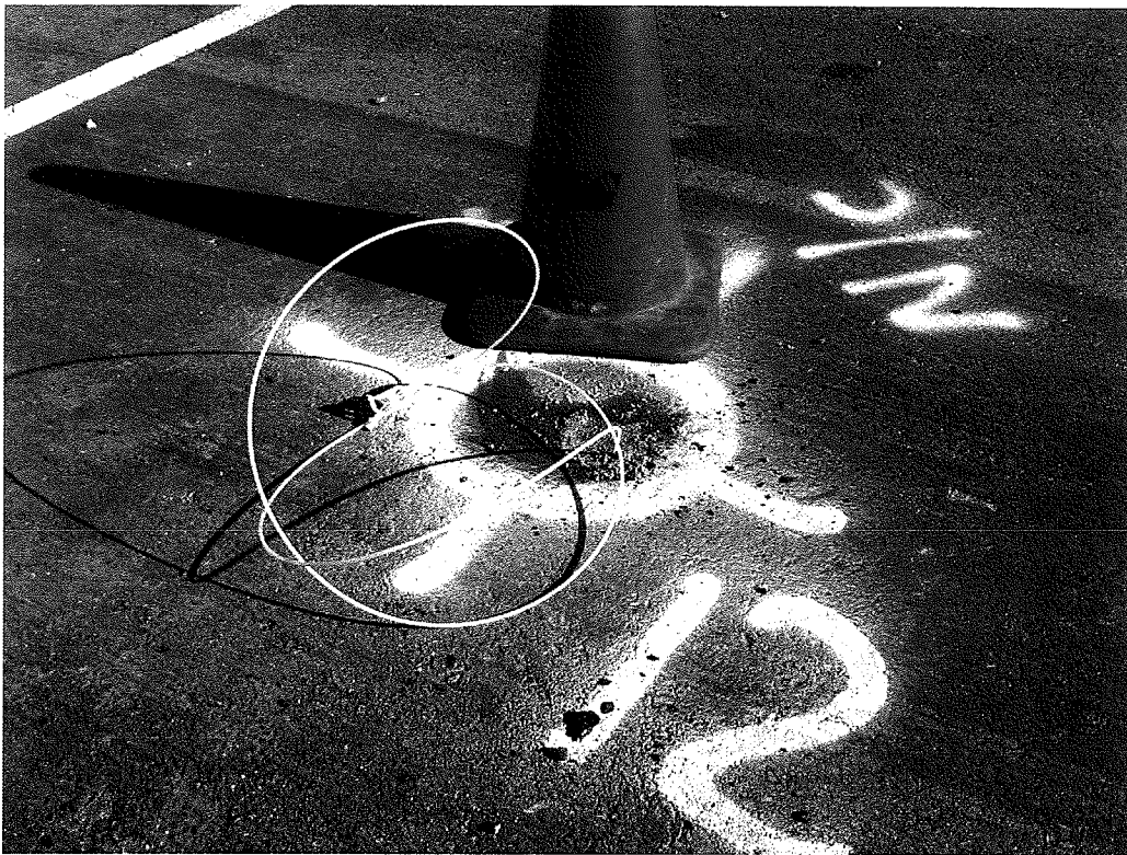
Photo 6, Bentonite seal placed and hydrated at soil-gas sampling location SG-12.
