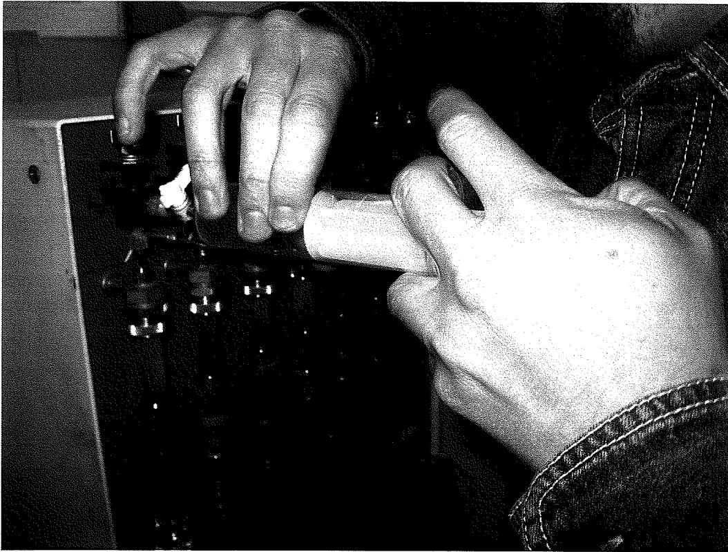
Photo 9, Chemist shooting soil-gas sample into analytical equipment inside mobile laboratory.
