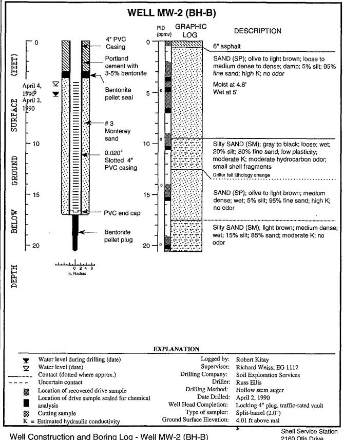
Well Construction and Boring Log - Well MW-2 (BH-B)
