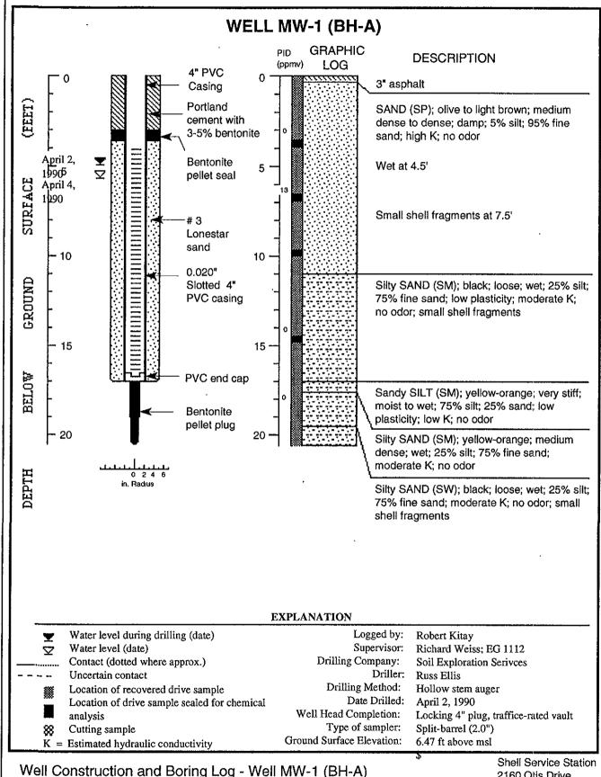
Well Construction and Boring Log - Well MW-1 (BH-A)
