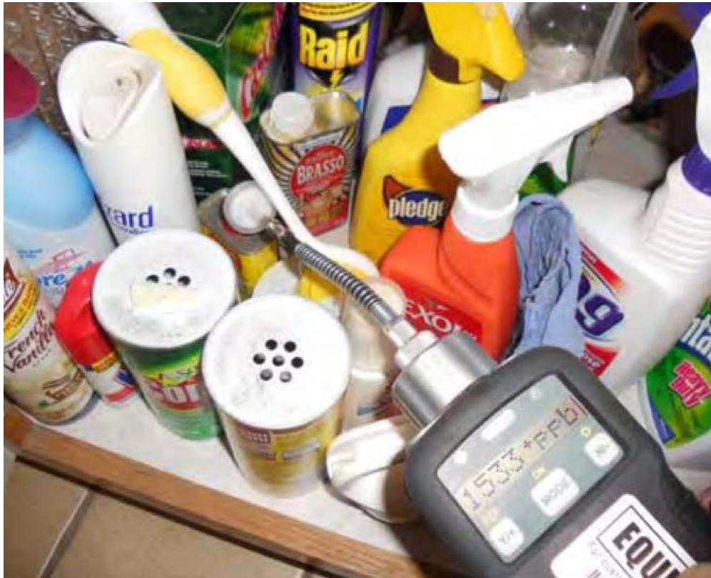
Special instrument to check for VOCs in household cleaning products.
