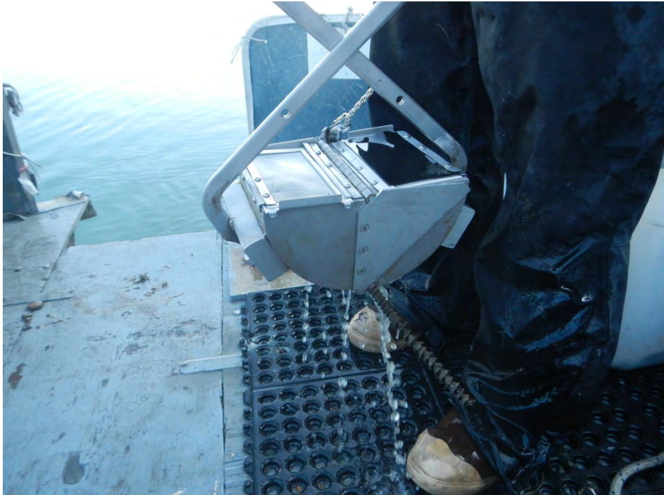
Photograph 13. SD-1 Metal Debris, Incomplete Closure (January 12, 2015)
