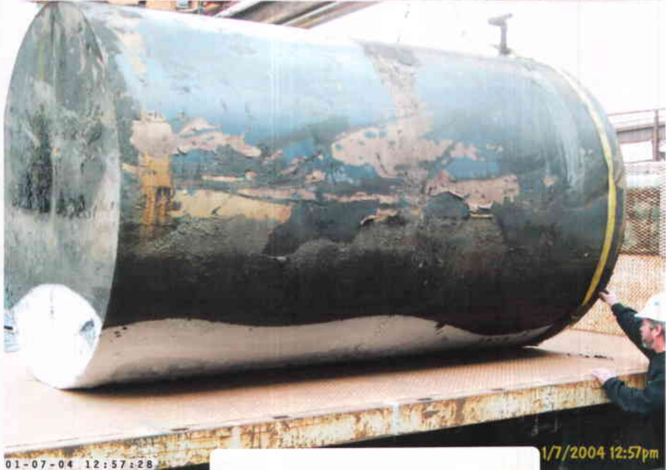
2000 gallon, single wall steel no apparent thru going holes
