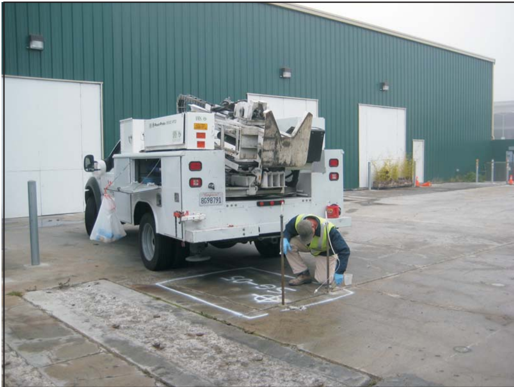
Photograph 9: TEG sealing deep probe at SG-05 with hydrated bentonite.
