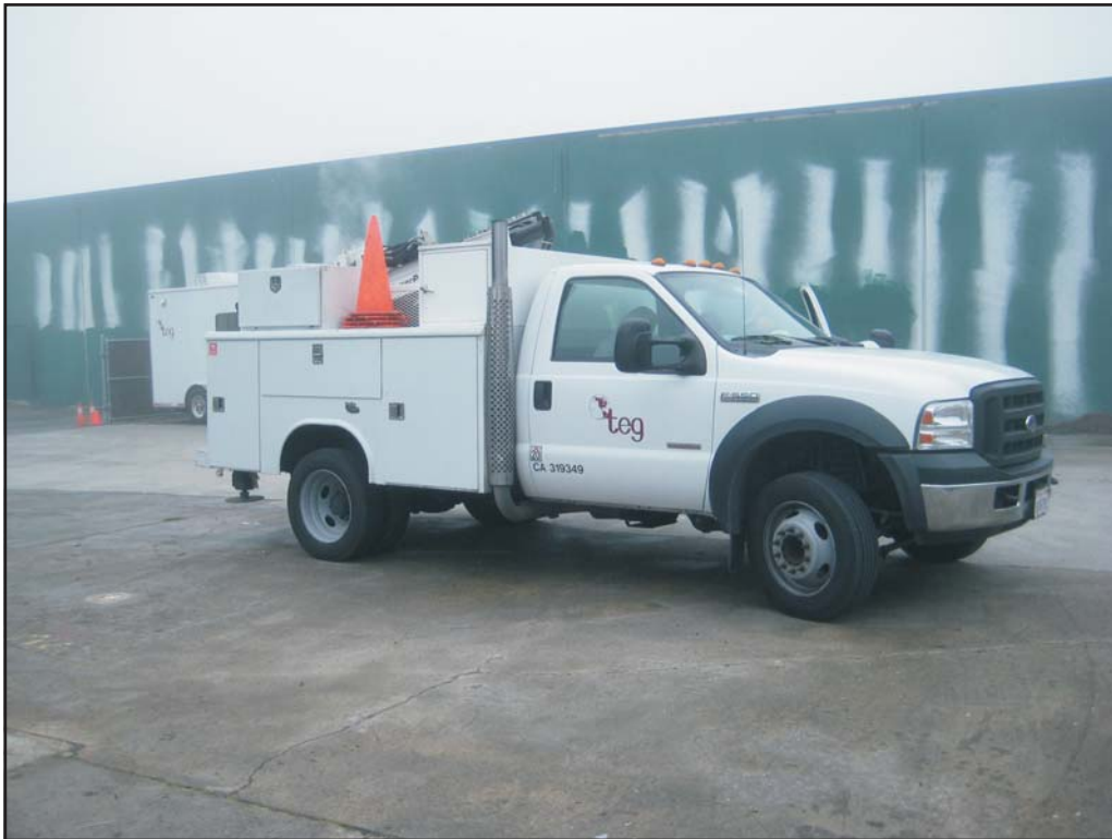
Photograph 1: TEG's direct-push rig.
