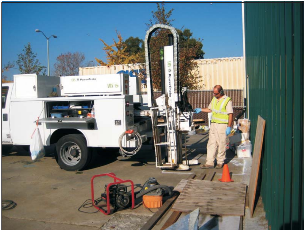
Photograph 27: TEG installing shallow probe at SG-02.
