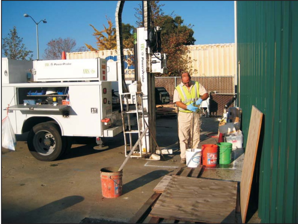
Photograph 31: TEG performing removal and decontamination of probes at SG-02.
