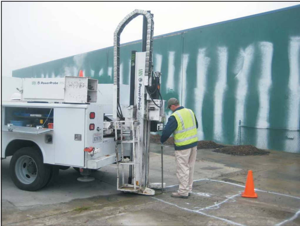
Photograph 3: TEG inserting tubing into vapor probe advanced at SG-04 to 5 feet bgs.
