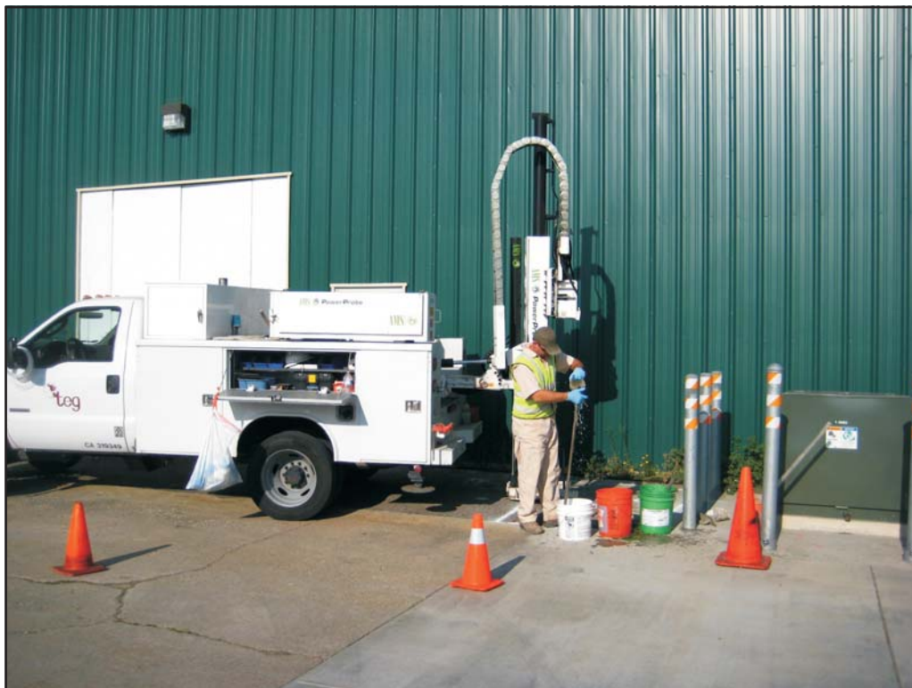
Photograph 24: TEG removing decontamination of probes from SG-01.
