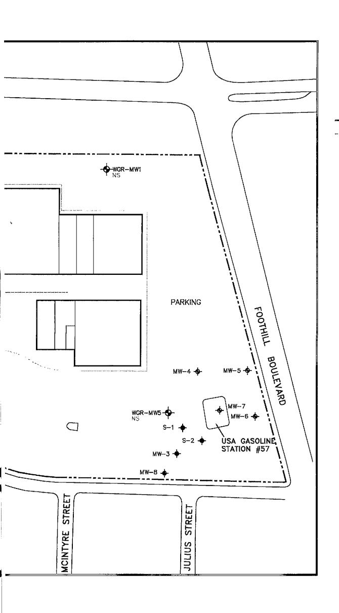
MW-1 Shallow Groundwater Zone Monitoring Well
