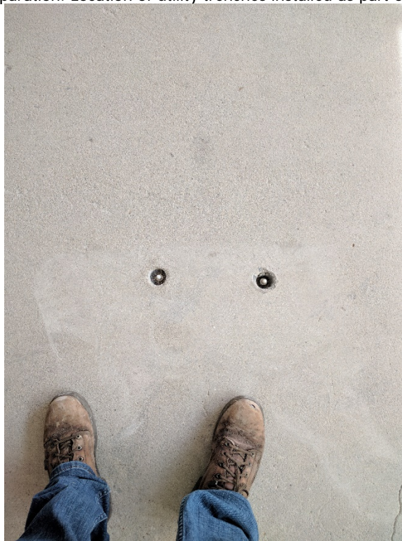
16. Representative cox-colvin sub-slab and soil vapor probe locations post abrasive surface preparation (03/11/2017)
