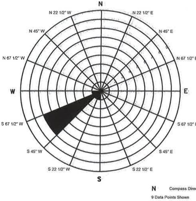
Rose diagram developed by evaluating the groundwater gradient direction from the quarterly monitoring data. Each circle on the rose diagram represents the number of monitoring events that the gradient plotted in that 22 1/2 degree sector. March 30, 2009 to November 23, 2011
