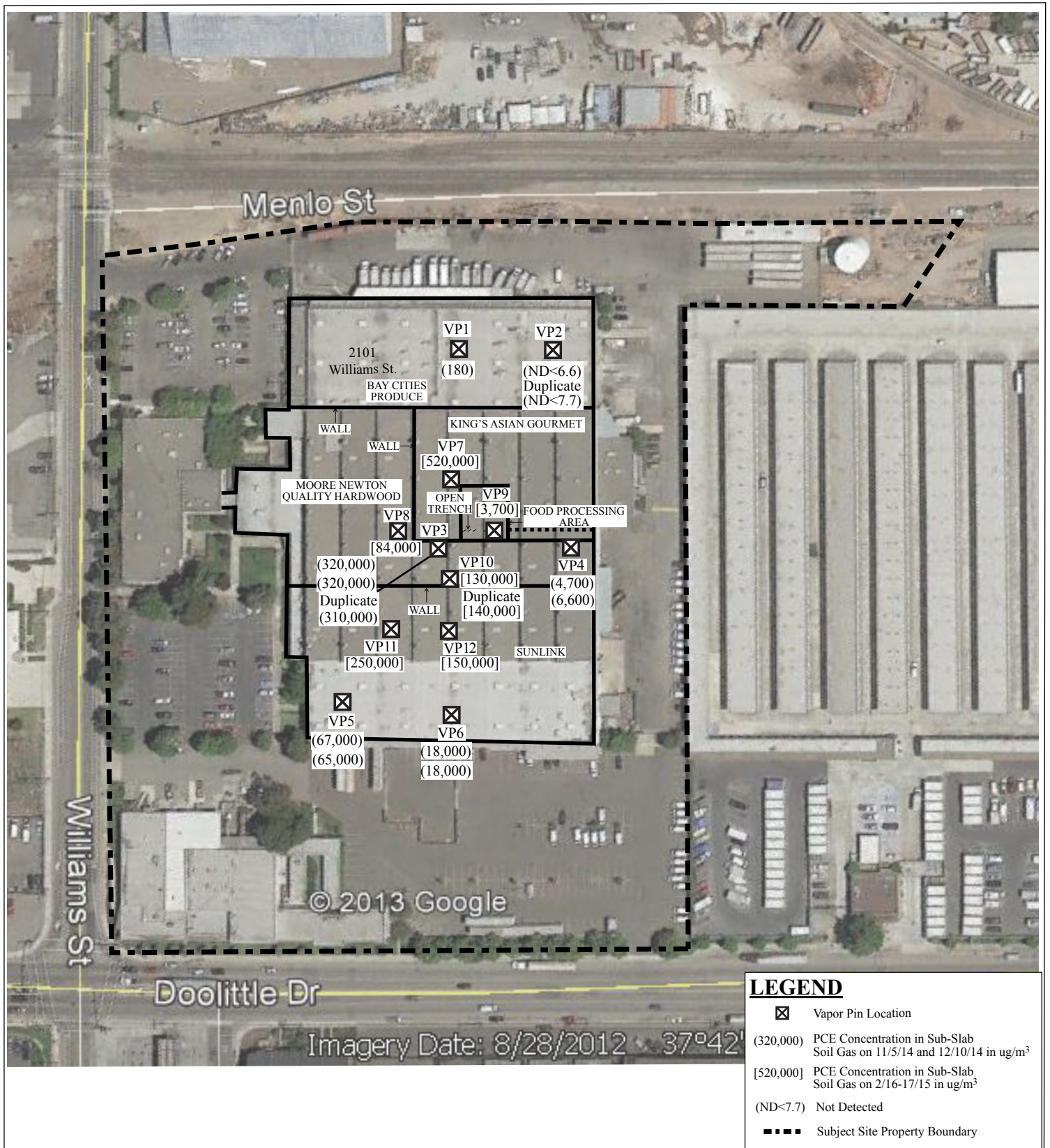
Figure 3 Site Plan Aerial Photograph Showing Vapor Pin Locations and PCE Sub-Slab Soil Gas Concentrations 2101 Williams Street San Leandro, California
