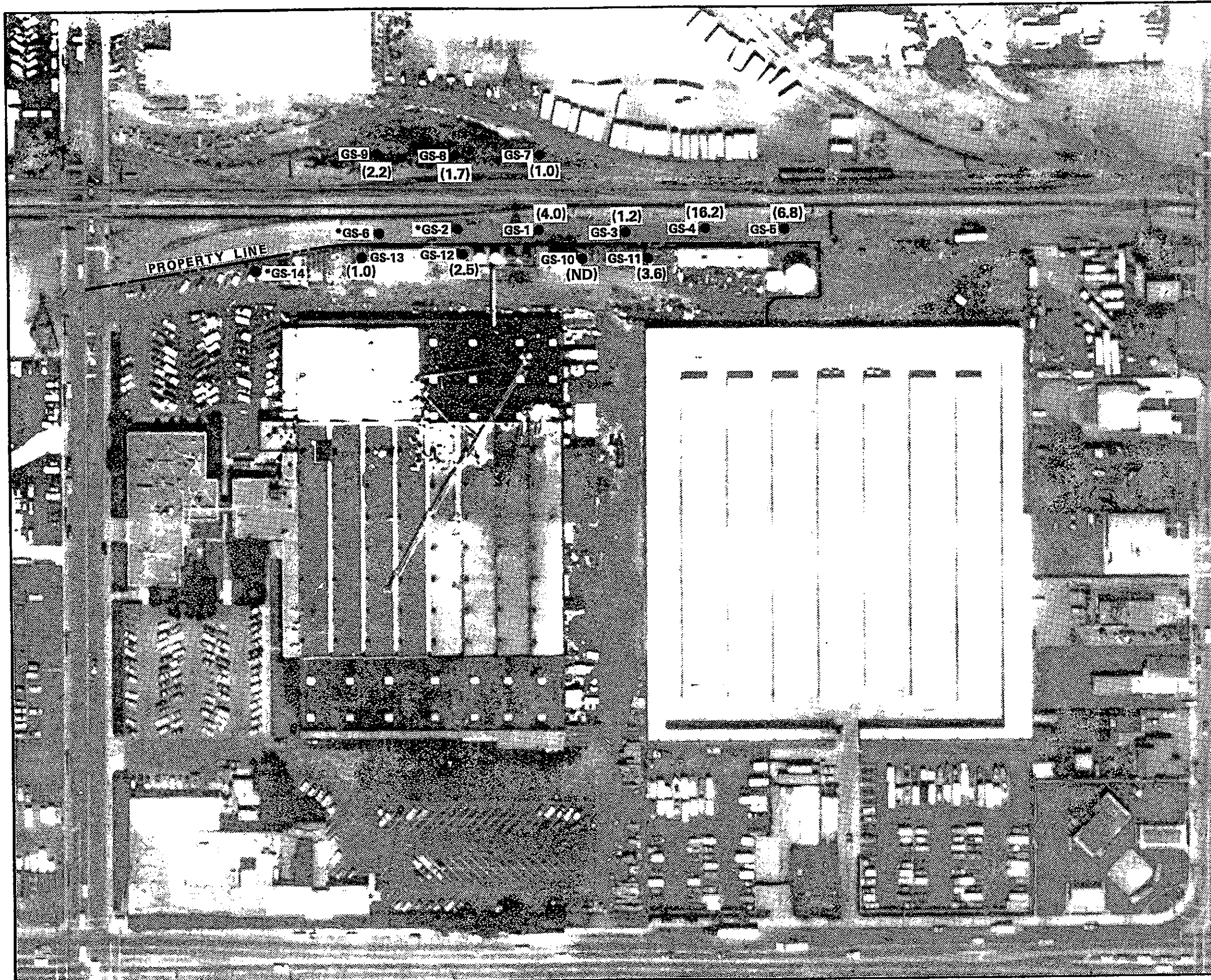
Figure 2 Distribution of DCE in Groundwater Survey Samples, James River Flexible Packaging Plant, San Leandro, California
