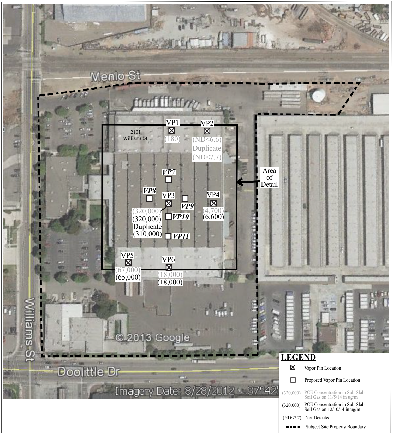
Figure X2 Site Plan Aerial Photograph Showing Vapor Pin Locations and PCE Soil Gas Concentrations 2101 Williams Street San Leandro, California
