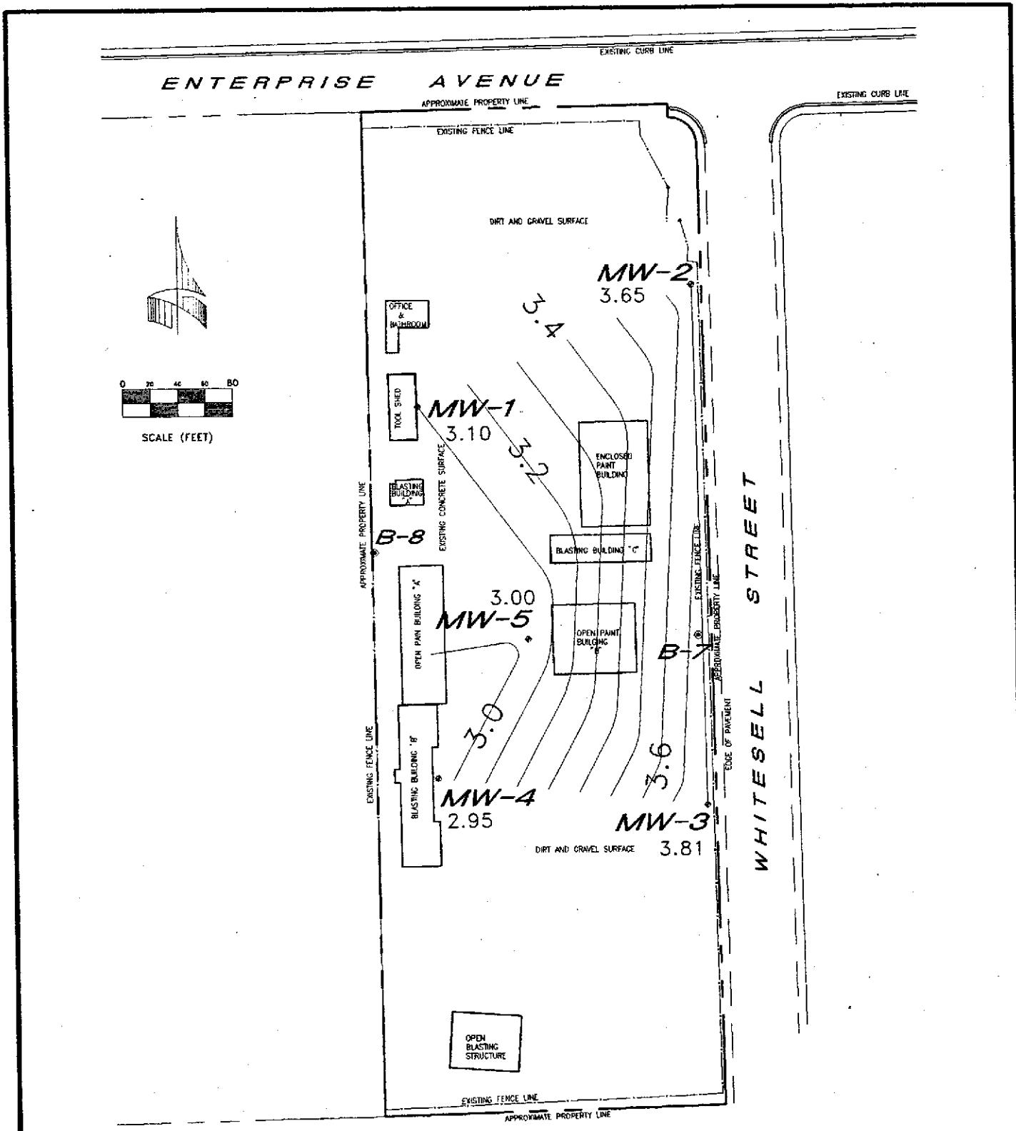
Well survey by Ron Archer, Civil Engineer, Inc., August 20, 1997. Top of casing elevations: MW-1 = 9.96; MW-2 = 8.86; MW-3 = 7.91; MW-4 = 8.47; and MW-5 = 8.86.
