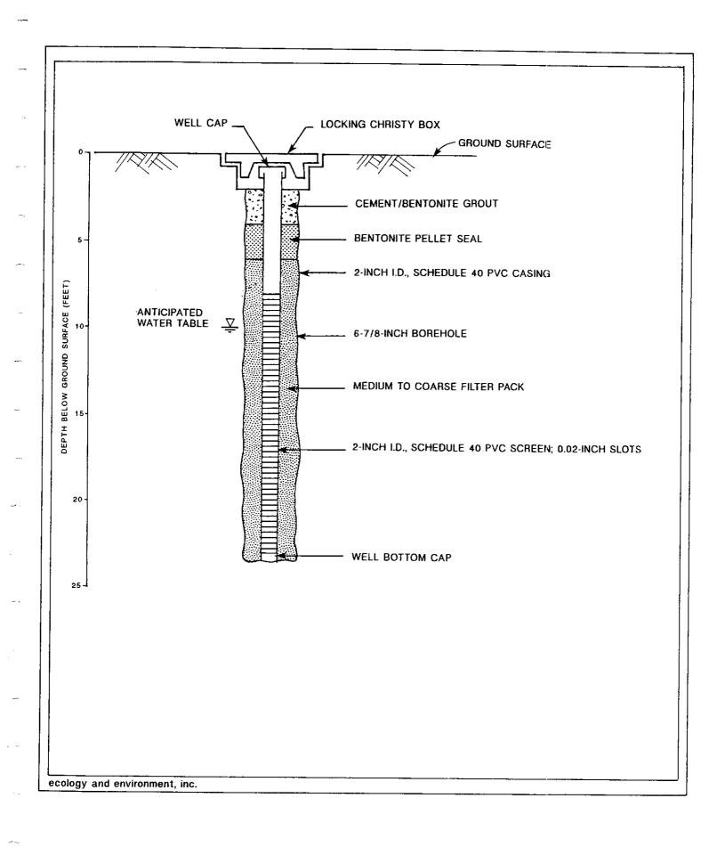
Figure 3.3 MONITORING WELL CONSTRUCTION DIAGRAM
