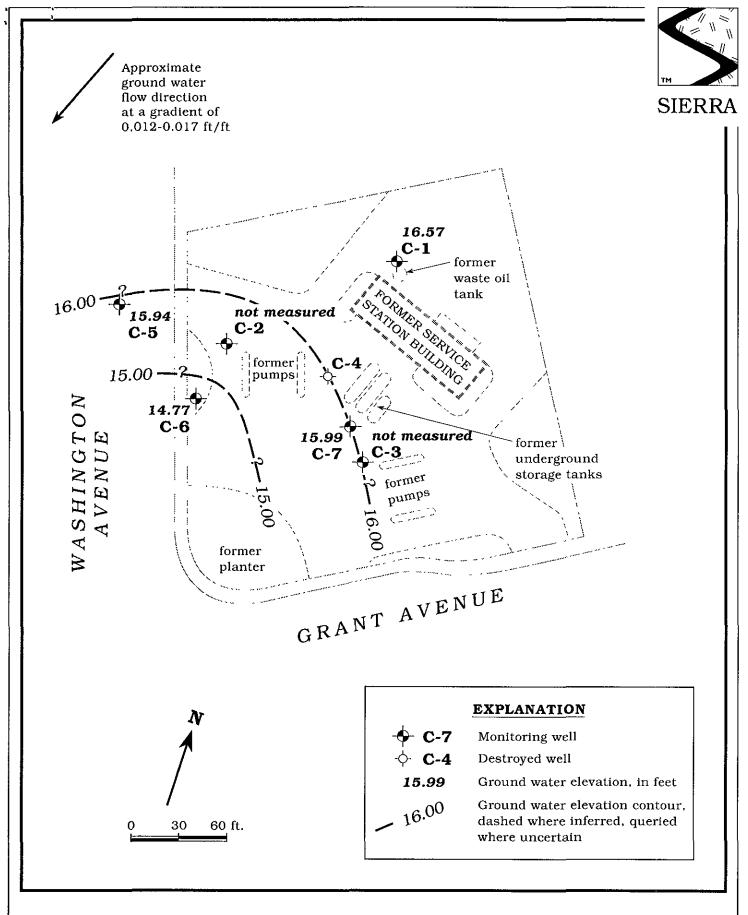
Figure 1. Monitoring Well Locations and Ground Water Elevation Contour Map - February 1, 1995 - Former Chevron Service Station #9-5630, 997 Grant Avenue, San Lorenzo, California
