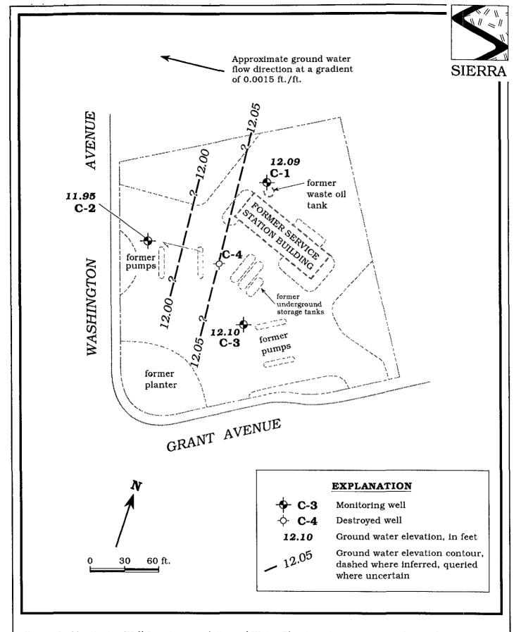
Figure 2. Monitoring Well Locations and Ground Water Elevation Contour Map - September 2, 1992 - Former Chevron Service Station #9-5630, 997 Grant Avenue, San Lorenzo, California
