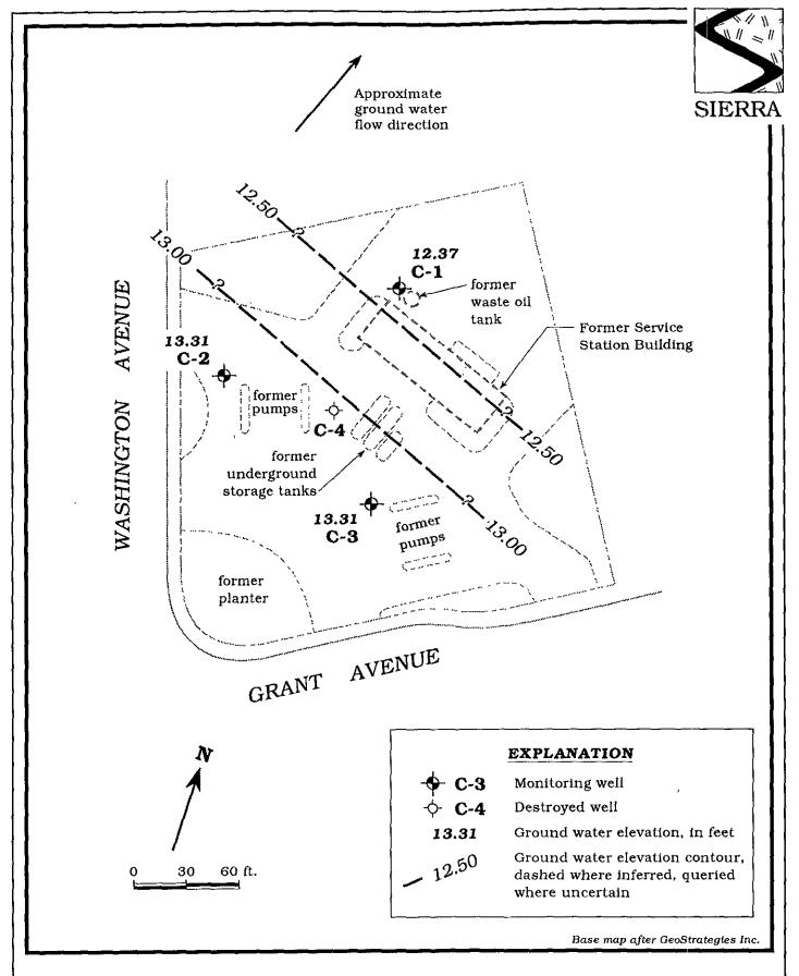
Figure 2. Monitoring Well Locations and Ground Water Elevation Contour Map - December 4. 1991 - Former Chevron Service Station #9-5630, 997 Grant Avenue, San Lorenzo, California
