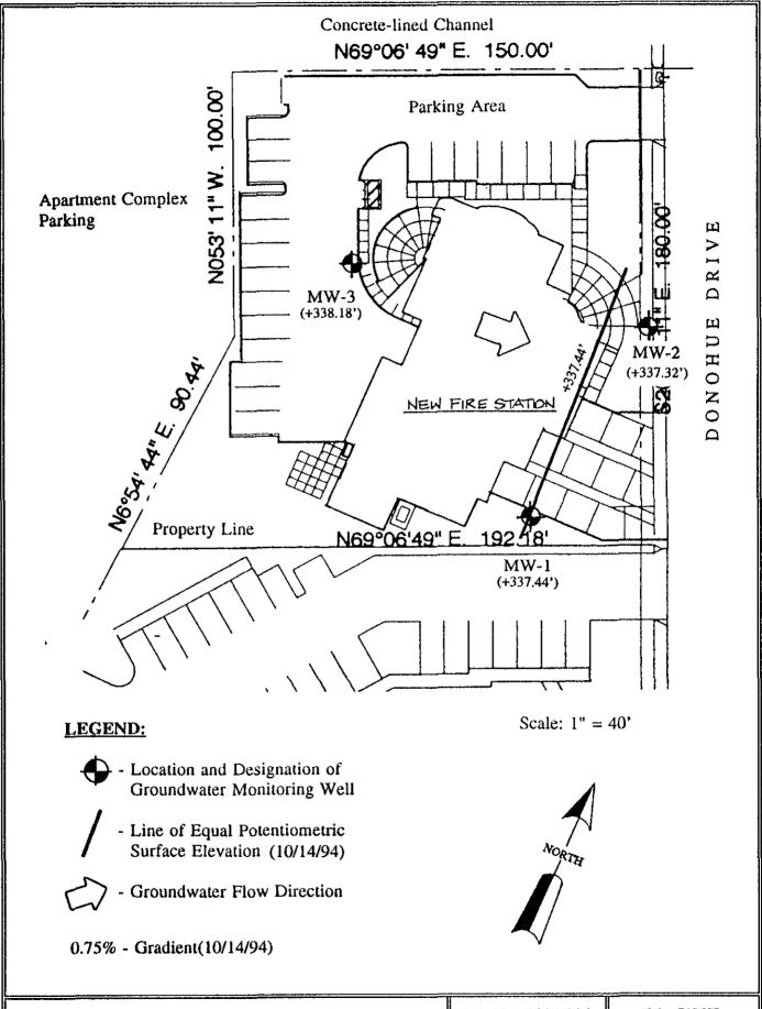
GROUNDWATER FLOW DIRECTION AND GRADIENT - 10/14/94
