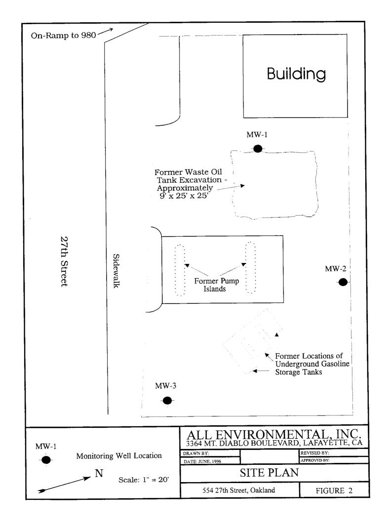
AEI drilled three soil borings and converted each boring into a groundwater monitoring well on June 22, 1995. This subsurface investigation included logging boreholes under the supervision of a Registered Professional Engineer, soil sampling and analyses, well development, and groundwater sampling and analyses.
