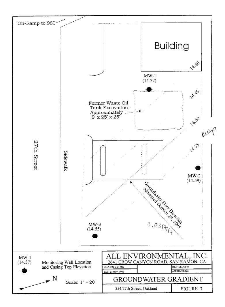
Groundwater was checked for sheen and free product prior to purging and sampling. No sheen or free product was observed. The samples were taken using a clean disposable bailer. Water was poured from the bailer into amber liter bottles and 40 ml VOA vials and capped so that no head space or visible air bubbles was within the sample containers. The samples were labeled and placed on ice in an ice chest for transportation to Priority Environmental Labs under chain of custody protocol for analysis.
