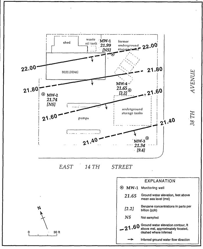
Figure 2. Monitoring Well Locations, Ground Water Elevation Contours, and Benzene Concentration in Ground Water - Oct. 4, 1995 - Shell Service Station WIC #204-5508-2709, 3750 East 14th Street, Oakland, California
