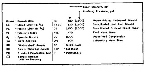
Note: All strength tests on 2.8" or 2.4" diameter sample unless otherwise indicated.
