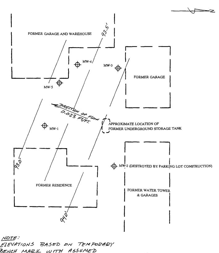
ELEVATIONS BASED ON TEMPORARY BENCH MARIL WITH ASSUMED ELEVATION OF 100.00 FT.
