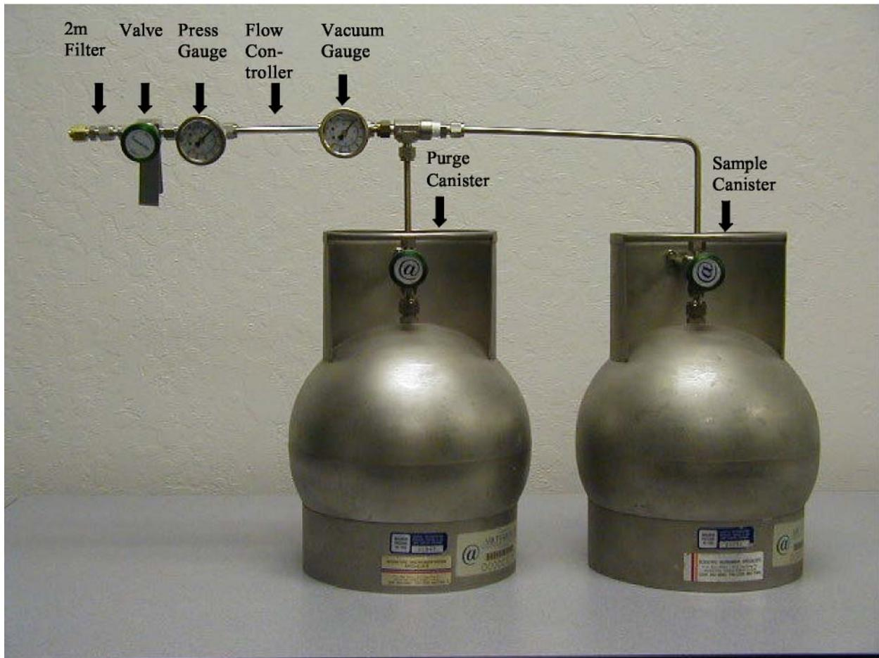
Figure 7. Typical Soil Gas Sample Collection Manifold
